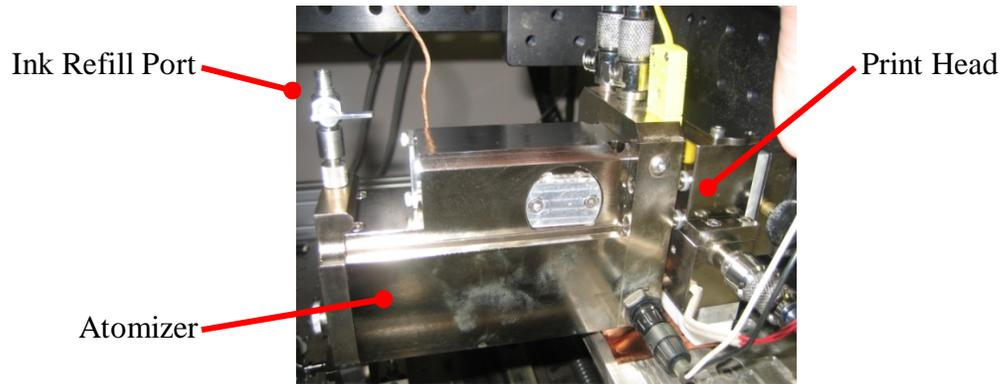
**Figure 7: Closely Couple Pneumatic Atomizer with Multiplexed Nozzles**
