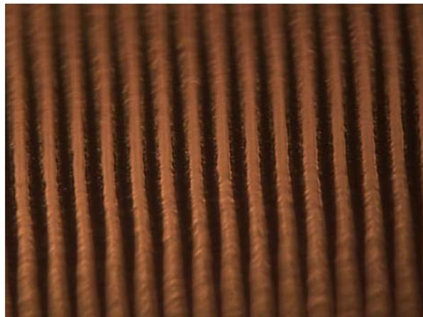
**Figure 6: Sub-75 micron pitch Silver interconnects**
