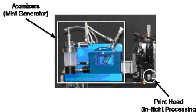
**Figure 1.** Schematic of the Aerosol Jet hardware and photo of the deposition head.
