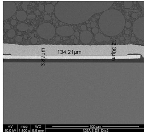
**Figure 5. Aerosol Jet Printed >10 $\mu$ m Thick Traces**
