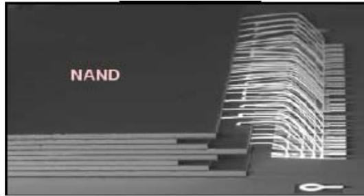
**Figure 3. Traditional Wire Bond Stacked Die**
