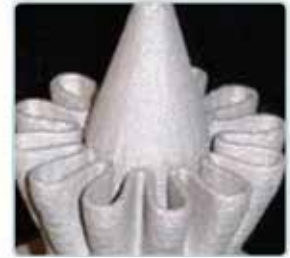
Exhaust Duct Fabricated by LENS System
