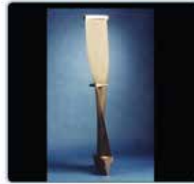
Compressor Blade Repaired by LENS System
