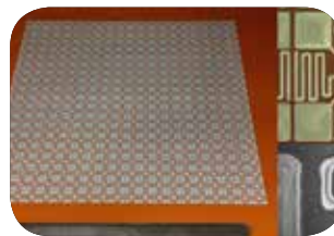
Fully Printed Phased Array Antenna Courtesy: Univ. Massachusetts, Lowell
