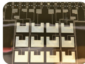
Phased Array Antenna
