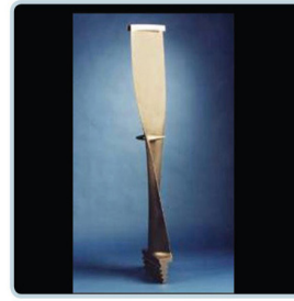
Compressor Blade Repaired by LENS System
