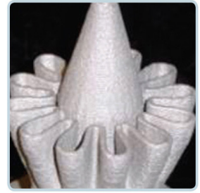
Exhaust Duct Fabricated by LENS System
